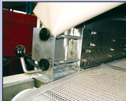
Air Flow Adjustment Louvers to Control Velocity and Direction of the Air Flow
