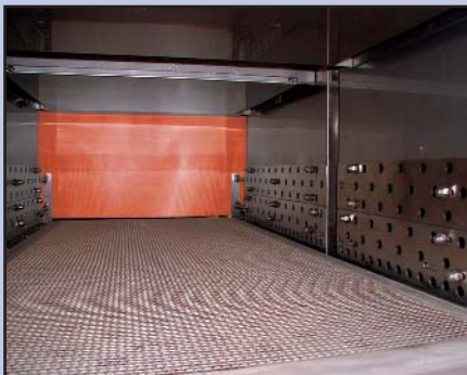
Tunnel Chamber with Mesh Belt
