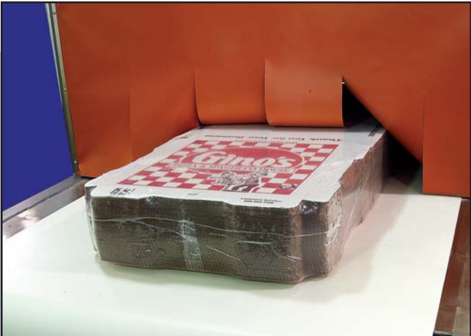
Wrapping Stacks of Corrugated Blanks
