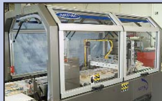
Gull wing doors provide unobstructed access
