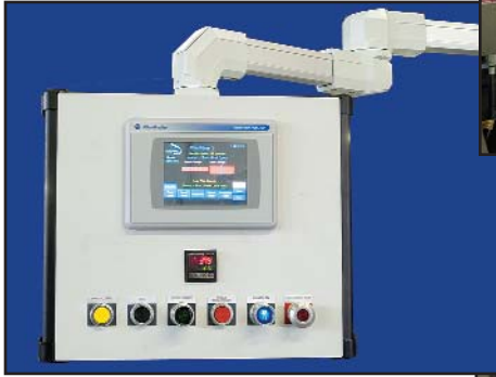
Operator controls can be reached from both sides of machine
