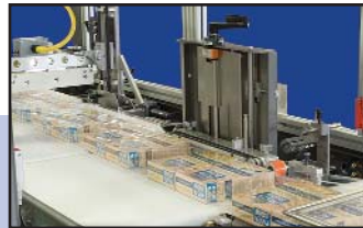
Side sealer with "Easy Open" feature for fast cleaning and inspection
