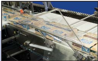
Patented film forming head for reliable transfer of products and fast easy film threading
